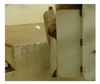
The flexi-reader panels are placed at 45° to each other to de-tune and reduce the read range. As a carcase pushes between the flexi-panels they re-tune, and proximity sensors allow the eartag EID to be read by the pre/post EID blocker. The pre/post EID blocker then checks the EID with a list of previous EID's recorded and only sends the ID if it is a new one.
