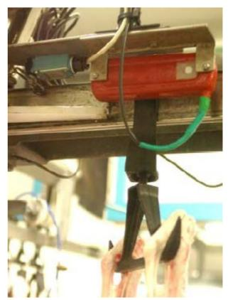
The HF transponder in the gambrel is read by an elongated SCL HF antenna connected to a HF reader.
