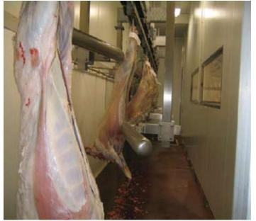
Figure 1. Six-module medium-voltage post-dressing stimulation system. The number of modules (electrodes) is determined by chain speed. With a faster chain, more modules are required to ensure only one carcase is on an electrode at any one time.
