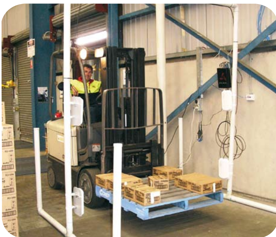
Above: Tagged CHEP pallets and reader at Linfox site.
