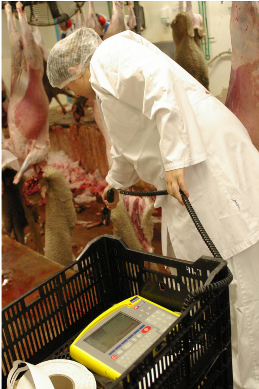
Manually reading eartag EID with grey Allflex stick reader connected to an XR3000 to obtain tracking number
