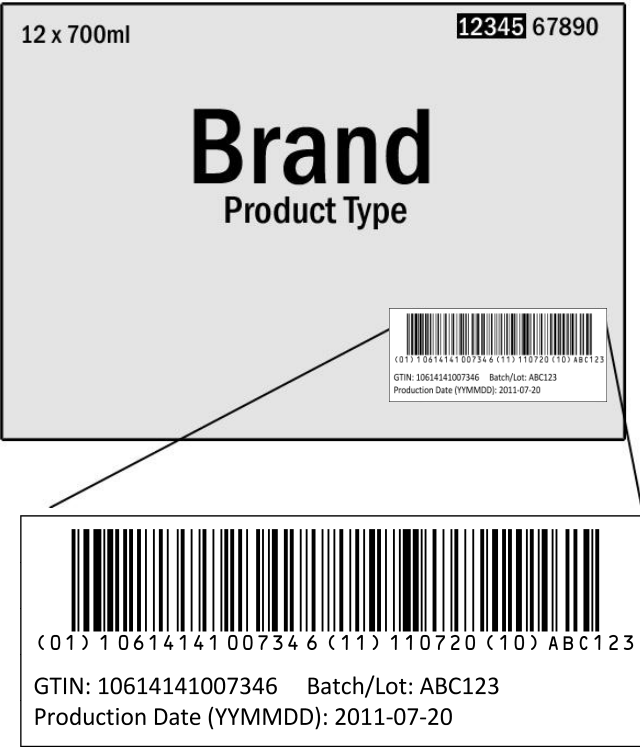
Sample case label showing use of GS1-128 barcode and human readable text to communicate GTIN (01), Batch/Lot Number (10) and Production Date (11)
