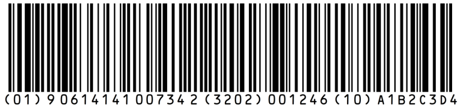
Figure 5 - Sample GS1-128 barcode with GTIN (01), Net Weight (3202), and Batch/Lot Number (10)
