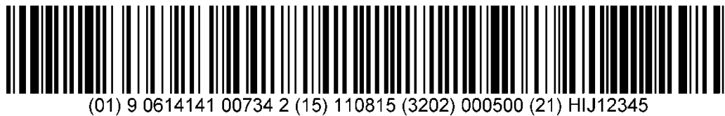
Figure 7 - Sample GS1-128 barcode with GTIN (01), Best Before Date (15), Net Weight (3202), Serial Number (21)
