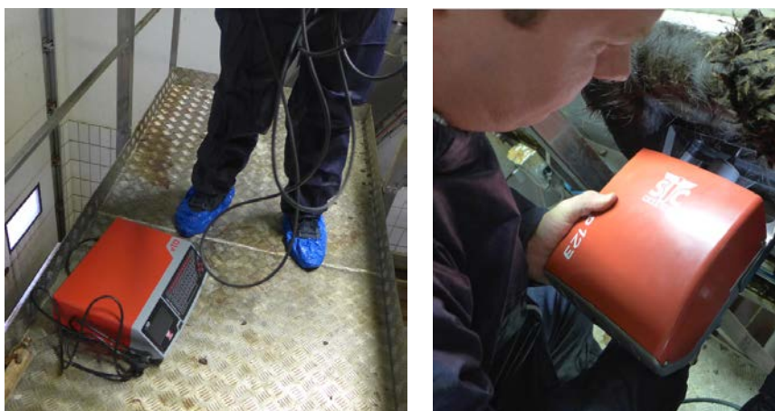
Figure 12. To the left: The stationary SIC Marking's e1 controller of the Dot Peening machine. To the right: The handheld part of the Dot Peening machine while testing on fresh hide. Photo: SINTEF Ocean.
