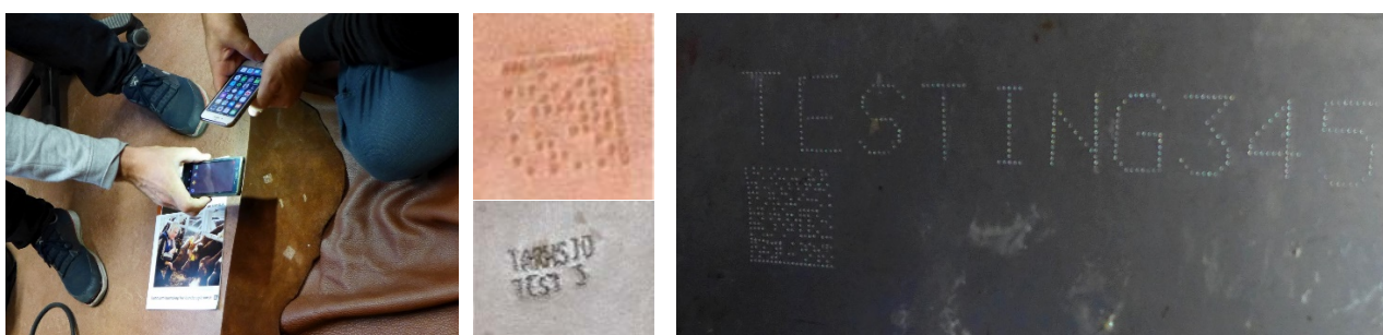
Figure 13. To the left: Hides were tested in the office prior to entering the facility and tagging fresh hides. Middle: Dot peening on hides after the tannery. Right: Text and QR code printed on the hides using Dot Peening. Photo: SINTEF Ocean.
