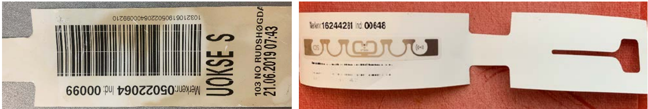
Figure 9. To the left is the hide tag used in production today. The right shows labels with glued RFID tag on one side. However, due to production errors the tags were glued to the wrong side of the labels. Photo: SINTEF Ocean.
