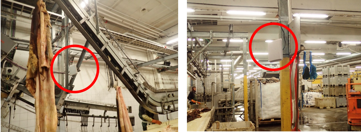
Figure 10. Antennas used at Skjeberg during the tests with RFID tagging of hide tags. Photo: Geir Vevele.
