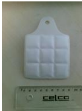
Tag B: "hang tag", broad-spectrum (860-960 MHz)
